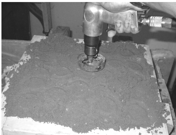
Figure III-14: Finishing the ramming
